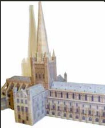
Traditional methods for constructing **prototypes for buildings** can be time consuming. Rapid prototyping of architecture using 3D printing can provide an efficient medium through which accurate coloured models may be produced.
